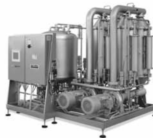
Ceramic Cross-flow filters, flowrate ranging from 200 to 15,000 gallons/h and over
